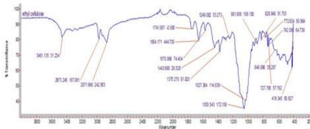
Figure 15: FT-IR spectra of Ethyl cellulose
